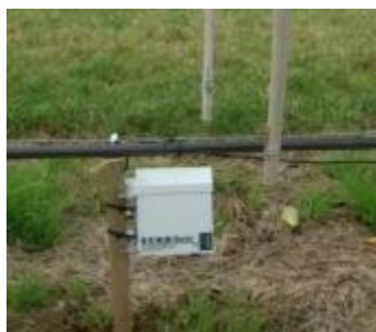
Figure 9. Rain gauge positioned under an emitter to record irrigation volumes in the concept pear orchard at EMR
