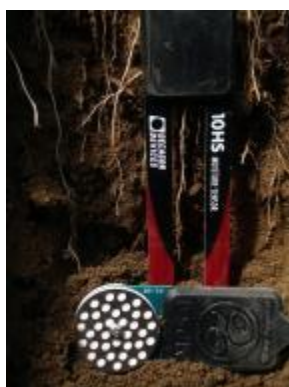
Figure 2. Decagon MPS1 probes and 10HS probes used to measure soil water availability and soil moisture content in the concept pear orchard at EMR
